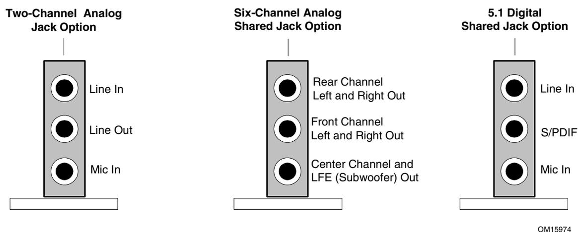
**Figure 3. Back Panel Audio Connector Options for Flex 6 Audio Subsystem**
